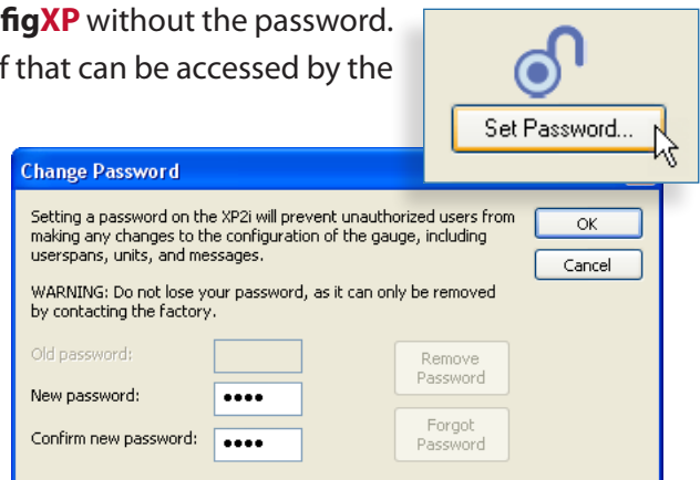
Figure 14 – Prevent unauthorized changes to a gauge with Password Protection.
